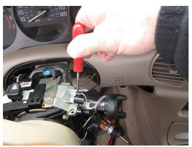
12) Remove the lock cylinder. This step may need to be performed before you can take the upper cover off on sime models. In order to do this you will need to located the access hole in the upper housing. Turn the ignition switch to the "Start" position with one hand. While inthat position, with the other hand, depress the pin inside this hole and slide the lock cylinder out.
