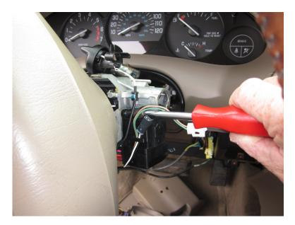
14) Remove the 2 bolts securing the ignition switch to the housing.
