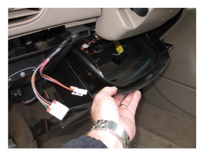
5) Remove the knee bolster panel. This is secured by 4 7mm bolts and 4 10mm bolts.
