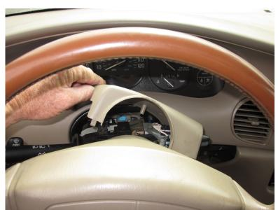
11) Remove the upper cover by pushing it towards the front of the car to release the front plastic lip from under the steering wheel.
