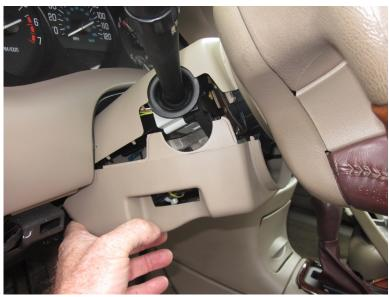
8) Remove the lower cover by pushing it towards the front of the car to release the front plastic hook tabs securing the upper and lower covers together.
