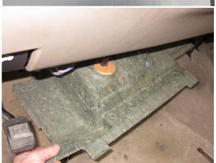
2) Remove the lower sound insulator panel to gain access. On some vehicles, there are multiple panels. You will need access between the kick panel and the center floor hump
