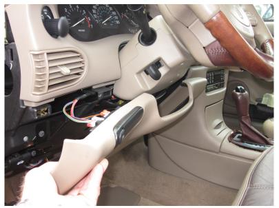
4) Remove the lower dash panel, On some models, the instrument cluster face panel will need to be removed first to gain access to hidden screws securing this panel. This model simply snaps off after 1 bolt on the bottom is removed.
