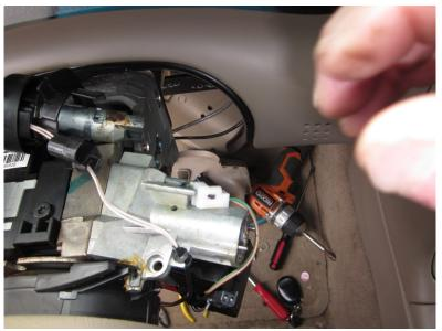
13) Remove the key warning buzzer contact. This is held in place by a plastic tab located on the inside of the contact. Depress the tab and rotate the contact assembly clockwise to release it.
