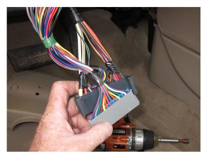
17) Split the connector by sliding the turn signal switch and wiper switch connectors out of the bulk connector. They are held in place by a small tab on the inside edge. Gently pry the tab while sliding the connectors apart.
