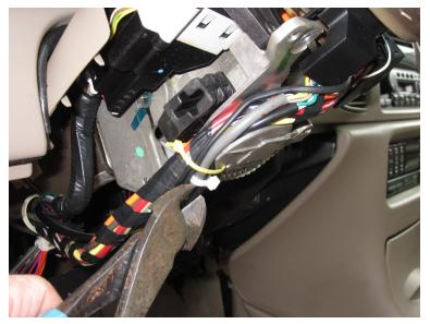
9) Cut the multiple ties straps securing the wire harnesses to the column and other harnesses
