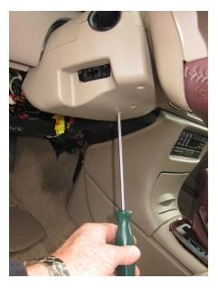
7) Remove the lower steering column shroud. Most GM vehicles have 2 20 torx bolts securing them to the column. This model simply snaps off after 1 bolt on the bottom is removed.
