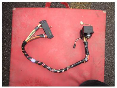
18) Remove the switch and harness from the car
