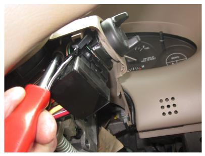
10) Remove the upper steering column shroud. Most GM vehicles have 1 inverted torx bolts securing the cover to the column. This bolt is hard to see, but is mounted as shown.
