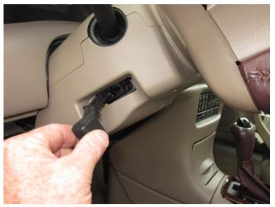
6) Remove the tilt release lever. This plastic lever snaps out of the housing by pulling firmly towards the door.
